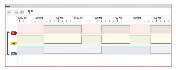
Logic Analyzer Capture of the NL (Normally Low), NH (Normally High), and TG (Toggle) outputs of LSVR Switch
