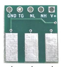
When the switch is in its inactive (non-pushed) state. The NH (Normally High) output is logic 1 and the NL/HS (Normally Low/Handshake) output is logic 0. Furthermore, the TG (Toggle) output powers up logic 1.
