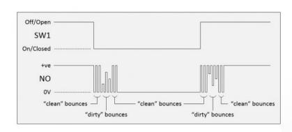
Switch bounce on an SPST-NO toggle switch (Image source: Max Maxfield)
