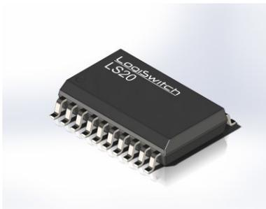
The LS10 Series of LogiSwitch debouncer/noise filter chips features low-impedance 25 mA totem-pole outputs for each channel. Outputs and inputs are of the same polarity and may be selected for use as active high or active low. The LS10 Series utilizes LogiSwitch's proprietary NoBounce technology resulting in a high level of noise immunity. Noise spikes of less than 20 ms duration are prohibited from initiating or terminating a cycle.
